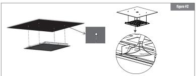
Connect the screw cap to the expanded nut of the ceiling. With power turned off at the breaker, connect power to driver based on the wiring diagram to complete the installation.
