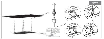
1. Position the expanded screws at one end of the cable on the ceiling and hook the other end of cable on panel.
