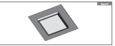
4. Push up luminaire the frame seamlessly.
