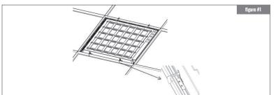
3. Fold the 4 protection brackets so they will be above the T-bar, as shown.
