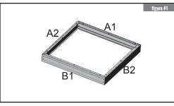
1. Fix A1/A2/B1/B2 with snap-in plastic comers making it a complete frame.
