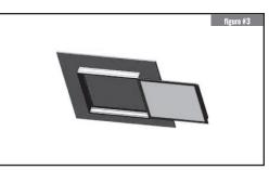
Slide partially the luminaire into the mounting frame, as shown. With power turned off at the breaker, connect power to drive based on the wiring diagram.
