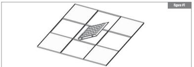
1. Remove the ceiling tile at an appropriate location where the product is to be installed and raise the product above the bar.
